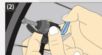
Engage to the valve of tire. Push down the lever to lock the valve.
