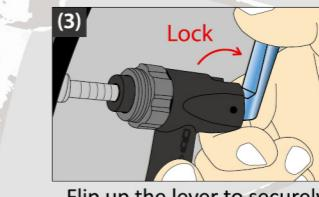
Flip up the lever to securely hold the valve, then inflate.
