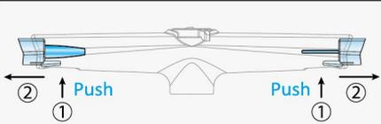
▲ Sliding handle plugs with ball needle and valve
